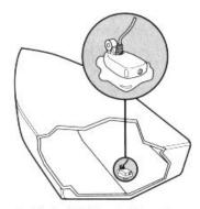
Inside the Hull Mounted Transducer
